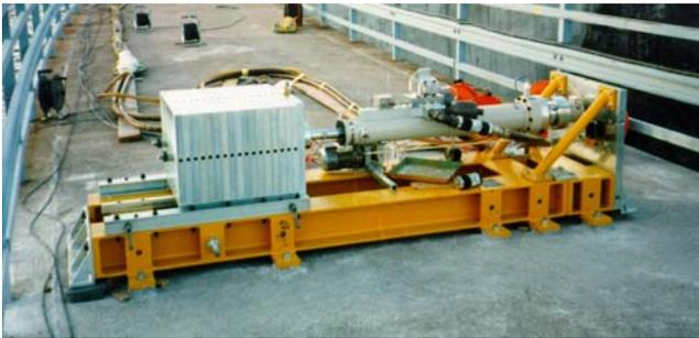
Fig. 3 The servohydraulic shaker
