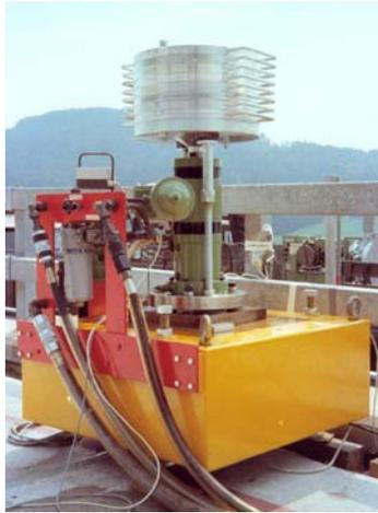
Figure 4 Servo-hydraulic shaker.
