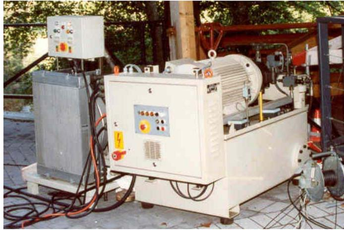
Figure 5 Hydraulic power pack used to drive the shaker shown in Figure 4.
