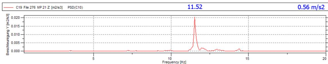
Figure 19: MP 21, Bus, right lane, 20 km/h. The shock absorbers in this suspension are probably quite worn. This results in the Bus exerting almost pure axle hop vibrations and exciting the cantilever at this quite high frequency even for using the right lane and at a comparatively low speed. The acceleration amplitude is quite high.
