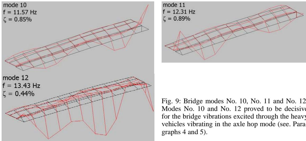
Fig. 9: Bridge modes No. 10, No. 11 and No. 12. Modes No. 10 and No. 12 proved to be decisive for the bridge vibrations excited through the heavy vehicles vibrating in the axle hop mode (see. Paragraphs 4 and 5).
