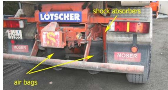
Figure 13: Rear axle air suspension.
