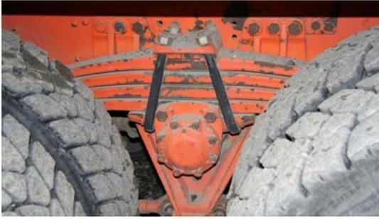
Figure 12: Rear axle steel suspension.
