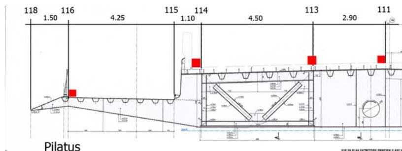
Figure 4: Ambient tests. Location of the four longitudinal measurement axes 111, 113, 114 and 116. Dimensions: meter.
