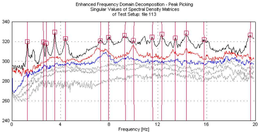
Figure 6: Ambient tests. EFDD-SVD diagram. For the sake of legibility this graphic covers the frequency range  $f = 0 \dots 20$  Hz only.
