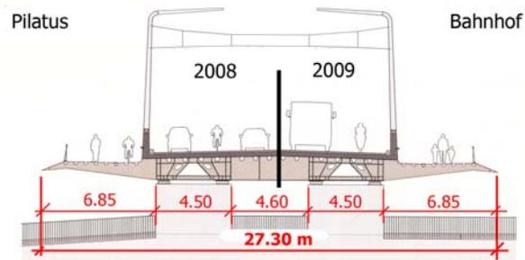
Figure 2: Langensand Bridge. Cross section. The paper covers tests performed on the Pilatus side half of the bridge (2008).
