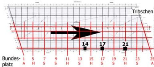
Figure 14: Location of the three 3D measurement points MP 14, MP 17 and MP 21. The driving direction is indicated.
