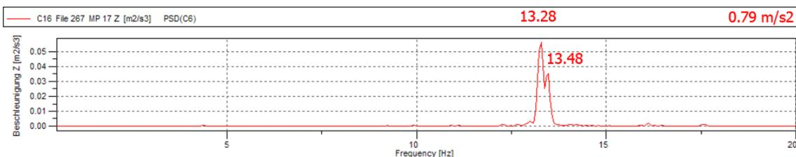
Figure 17: MP 17, Air suspended vehicle, left lane, 40 km/h. Driving in the left lane at a relatively high speed results in a nice excitation of cantilever mode No. 12. Although the modal amplitude in the driving lane is quite small, coincidence with frequency and the low modal damping lead to a maximum acceleration level in MP 17 where the modal amplitude is maximum.
