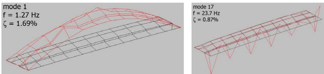
Figure 7: Modes No. 1 and No. 17 illustrating the bandwidth in frequency and shape of this bridge.
