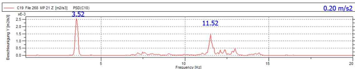
Figure 16: MP 21, Air suspended vehicle, right lane, 20 km/h. Right lane means: driving on the box girder. Global modes without a node in MP 21 (3.52 Hz) are more likely to be excited than local cantilever modes (11.57 Hz). The maximum amplitude (indicated in the graphic's top right hand corner) is comparatively small (0.2 m/s<sup>2</sup>).
