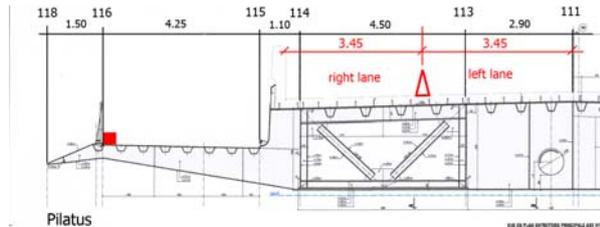
Figure 15: Location of the measurement points in the cross section (red square); situation of the two driving lanes.
