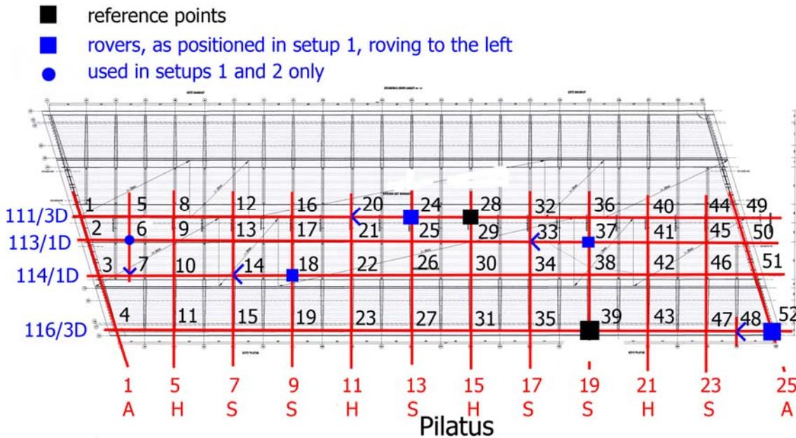
Figure 5: Ambient tests. Instrumentation layout.
