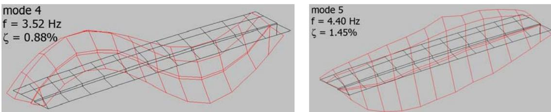
Figure 8: Bridge modes No. 4 and No. 5. These two modes proved to be decisive for the bridge vibrations excited through the heavy vehicles in the body bounce mode (see. Paragraphs 4 and 5).
