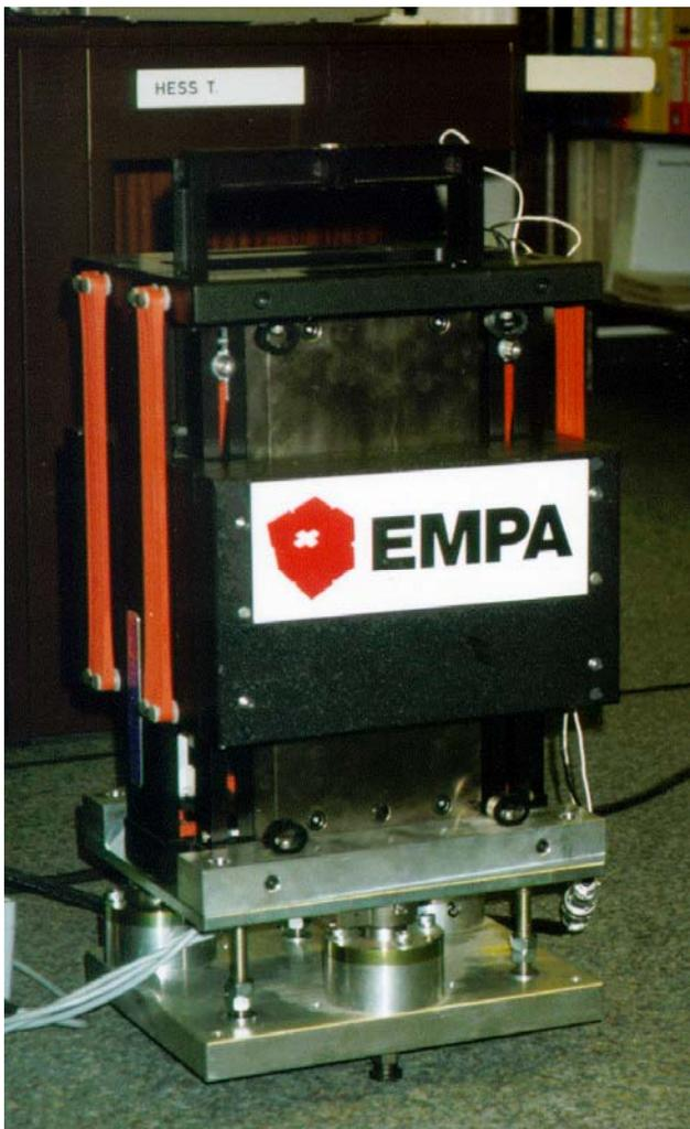
Fig. 5 The electrodynamic vibration generator.
