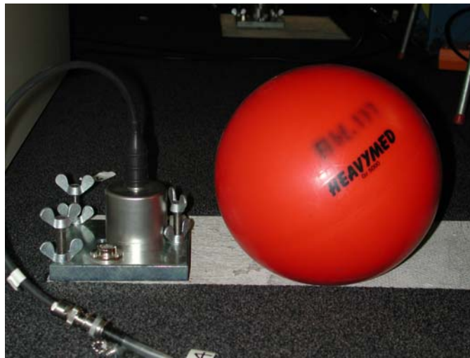
Figure 4: The medical ball used to excite the slabs and one of the accelerometers used to measure the slab response.
