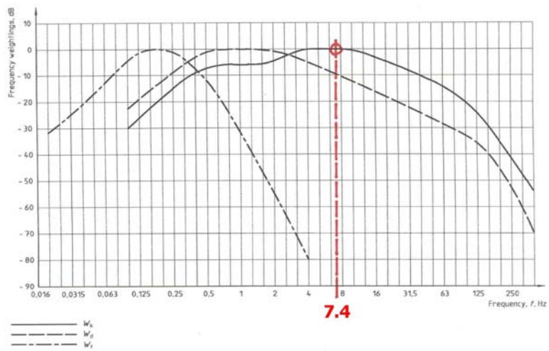
Figure 17: Frequency weighting curves as given in [4]. W_k (solid line) applies for vertical movement.
